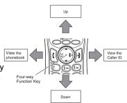
information. To use this four-way key, place your thumb over the key on the station and move to the four positions to get the feel of how it moves and operates.
